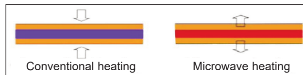
Fig. 1. Volumetric microwave heating and conventional surface heating
